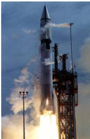
**The Atlas Centaur launch system. ARPA funded the development of the LH<sub>2</sub>/LOX Centaur upper stage, as a high performance stage necessary to lift heavy payloads. Combined with the Atlas and Titan boosters, Centaur was the upper stage for launches of probes to Mercury, Venus, Mars, Jupiter, Saturn, Uranus, and Neptune. Centaur continues to serve as the United States' most powerful upper stage.**
